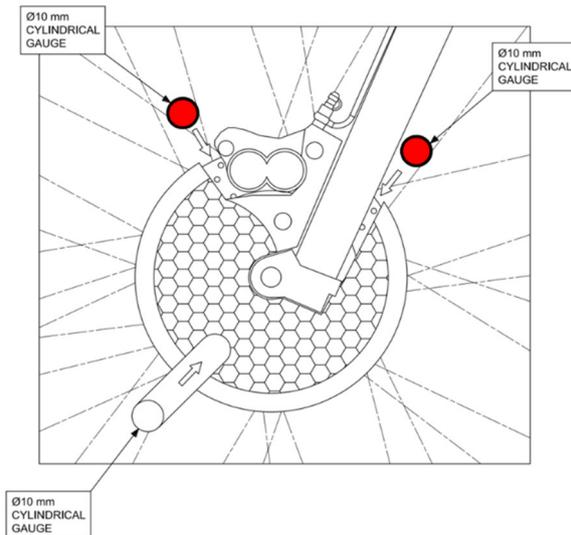
Figure 8 : Front brake disk protective cover
