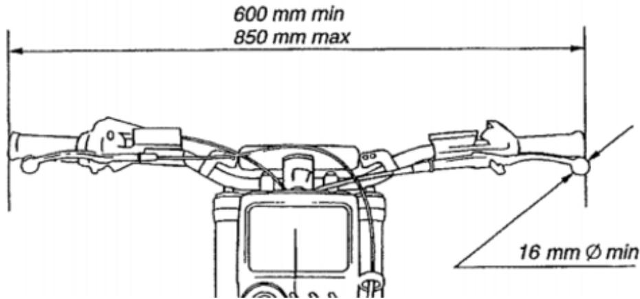
Figure 1 : Handlebar length
