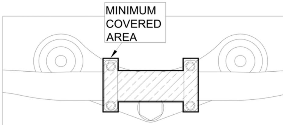
Figure 2 : Handlebar covering
