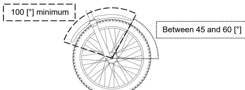
Figure 10 : Front mudguard position
