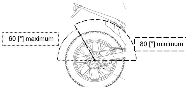
Figure 11 : Rear mudguard position
