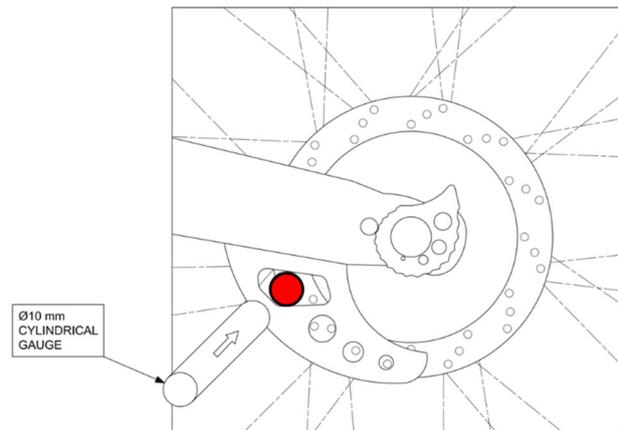
Figure 9 : Rear brake disk protective cover
